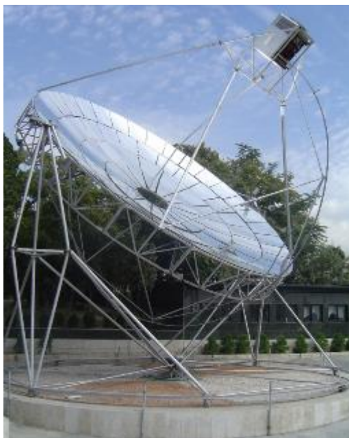
10kW Solar Dish/Stirling Engine System in NRI, Iran
