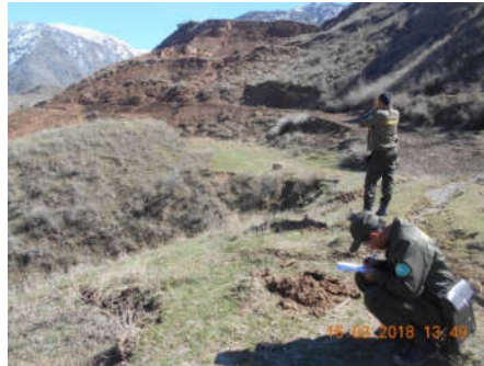
Measurement of landslide parameters with an electronic distance metre
