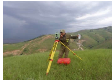
Topography of landslides using an electronic total station
