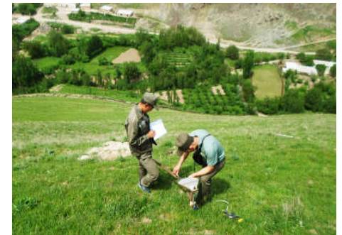
Measuring the opening of landslide cracks using a strain gauge
