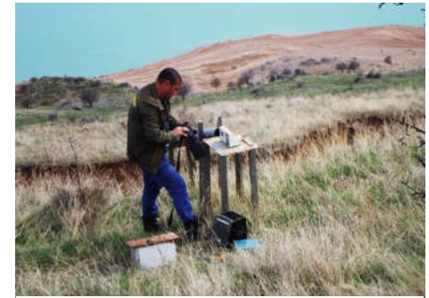
Landslide displacement measurement using an electronic extensometer
