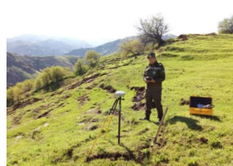
Landslide dislocation measurements using a GPS receiver
