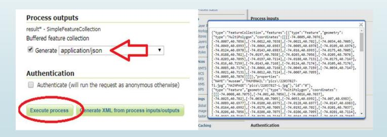
Use the "Generate XML from Process Inputs/Outputs" option to generate a request based on an XML file.
